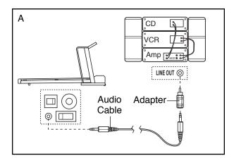
B. Plug one end of the audio cable into the jack on the front of the treadmill near the power cord. Plug the other end of the cable into the included adapter. Plug the adapter into an RCA adapter (available at electronics stores). Next, remove the wire that is currently plugged into the LINE OUT jack on your stereo and plug the wire into the unused side of the RCA adapter. Plug the RCA adapter into the LINE OUT jack on your stereo.
